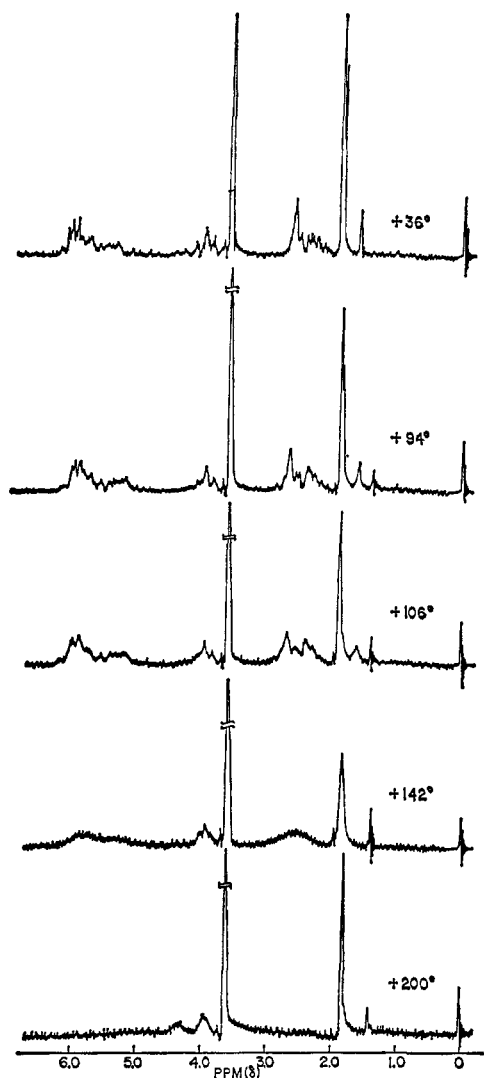
Figure 6. 60-MHz nmr spectra of 13 in \text{Cl}_2\text{C}=\text{CCl}_2 solution at 36, 94, 106, 142, and 200°. The sharp peak at \delta 1.39 is due to an impurity that could only be removed with great difficulty.
